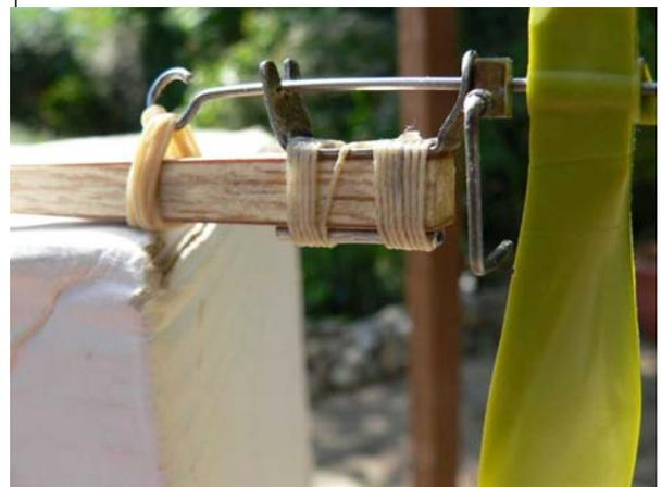
Fully adjustable for down and side thrust. The prop is replaceable and it's got that funny freewheeler. Also the U/C is removable. Ummm. That's it really. Oh yes, the band is just to stop the shaft flopping, it's NOT the motor!
