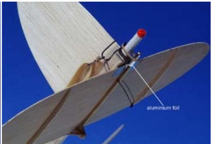
So far as I can make out, he's put the snuffer tube inside the 1/4" square fuselage stick. Clever.
