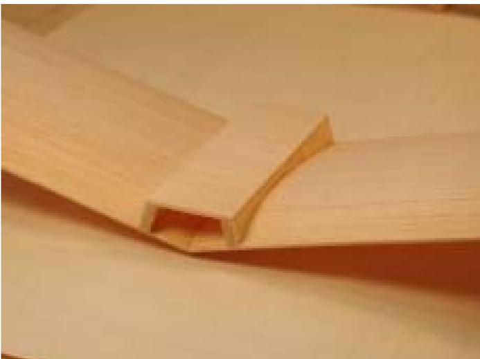
This modification also helps to avoid warps that can very easily creep into a flat, flexible surface. The picture from Pat Seale in Wisconsin shows the modifications. (ed's note, I've done this, and also included pegs to rubber band the wing on)
