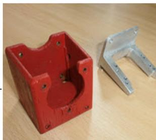
Motor mounting holes in the horse collar are 3mm. Spaced (surprisingly for a Czech motor)
