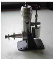
The only possible snag is that it is not beam mounted, and requires either a metal mount as shown here, or , (as recommended in the instructions,) a ply firewall.
