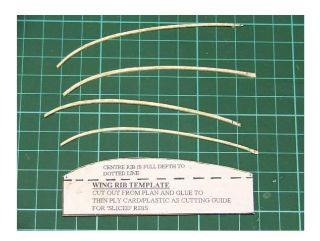
Gluing the ribs to the LE and TE is a tricky business, make sure the fit is accurate or they tend to break away as you handle and cover the wing. You can use super glue, it is fast but it can get out of control. Next one I am using aliphatic as it is easier to sand.
