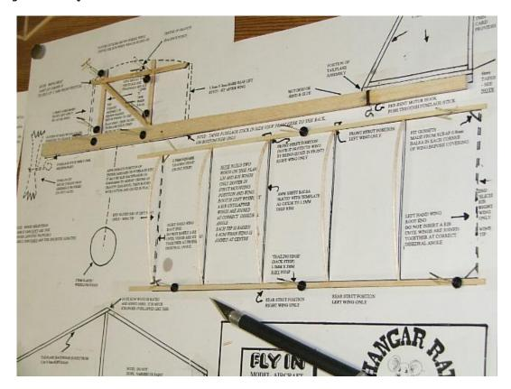
Covering the surfaces with tissue is straight forward if you use that paper glue in a stick. Put the glue on the framework then work the tissue on with your fingers. The tissue used here was with the kit, is light and a bit crinkly. I don't know enough about tissue to know the correct name but it's like shoe box or wrapping tissue from the newsagents.
