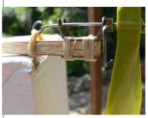
Fully adjustable for down and side thrust. The prop is replaceable and it's got that funny freewheeler. Also the U/C is removable. Ummm. That's it really. Oh yes, the band is just to stop the shaft flopping, it's NOT the motor!
