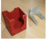
Motor mounting holes in the horse collar are 3mm. Spaced (surprisingly for a Czech motor)
