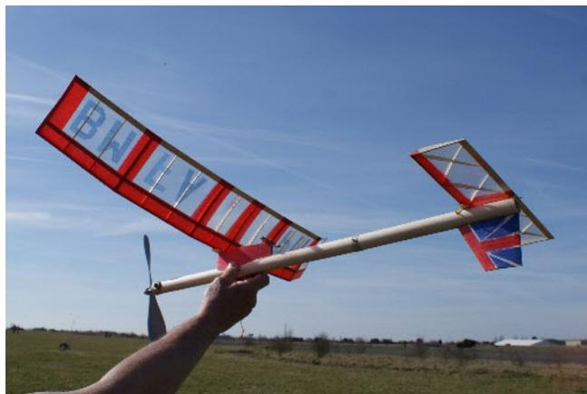
**At North Luffenham the day after,** Dave Bent demonstrated the “Tumbling Pigeon” d/t system: t.e of wing lifts, model summersaults & impersonates a shot pigeon, or a very sick duck. Comes down well: worth considering for lightweight models. Model is o/d P30
