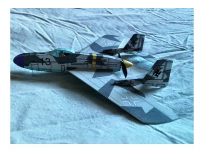
**Rob Smith is at it again** (again.) Powered by cheap quadcopter brushed motors (acquired from Amazon.) Power source by super capacitors. (Maplin.) As with other similar models these little masterpieces are built from balsa and D\*pron & covered with preprinted layout paper. Design by CAD.
