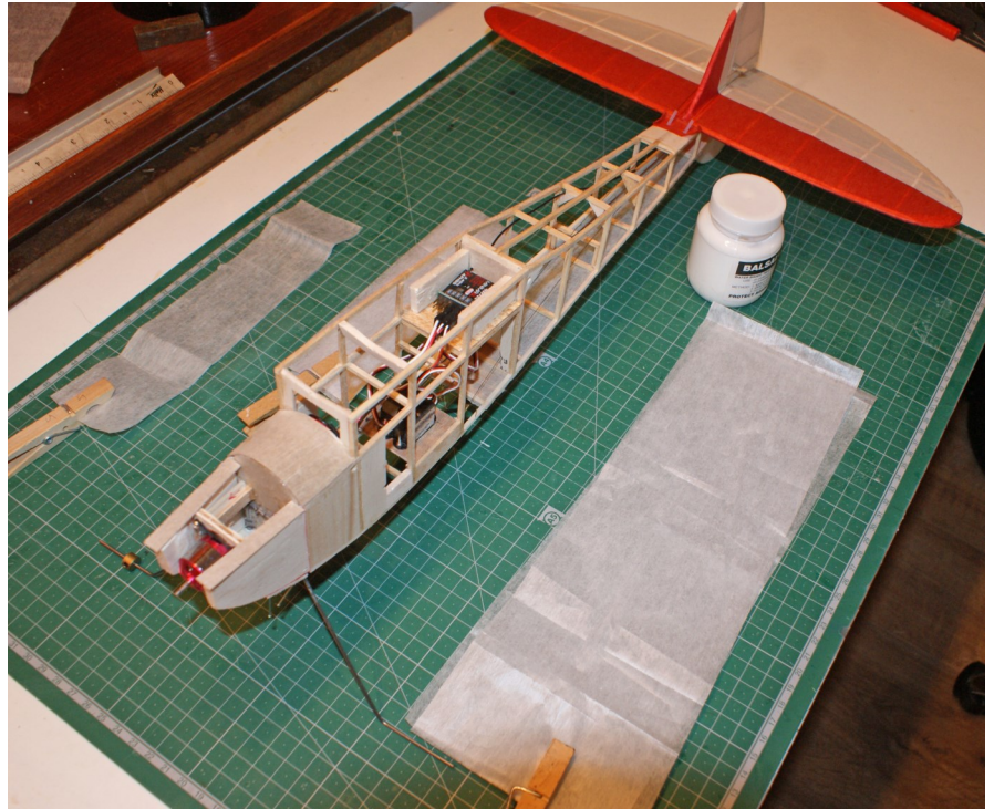
The Bantam fuselage awaits Polyester covering
