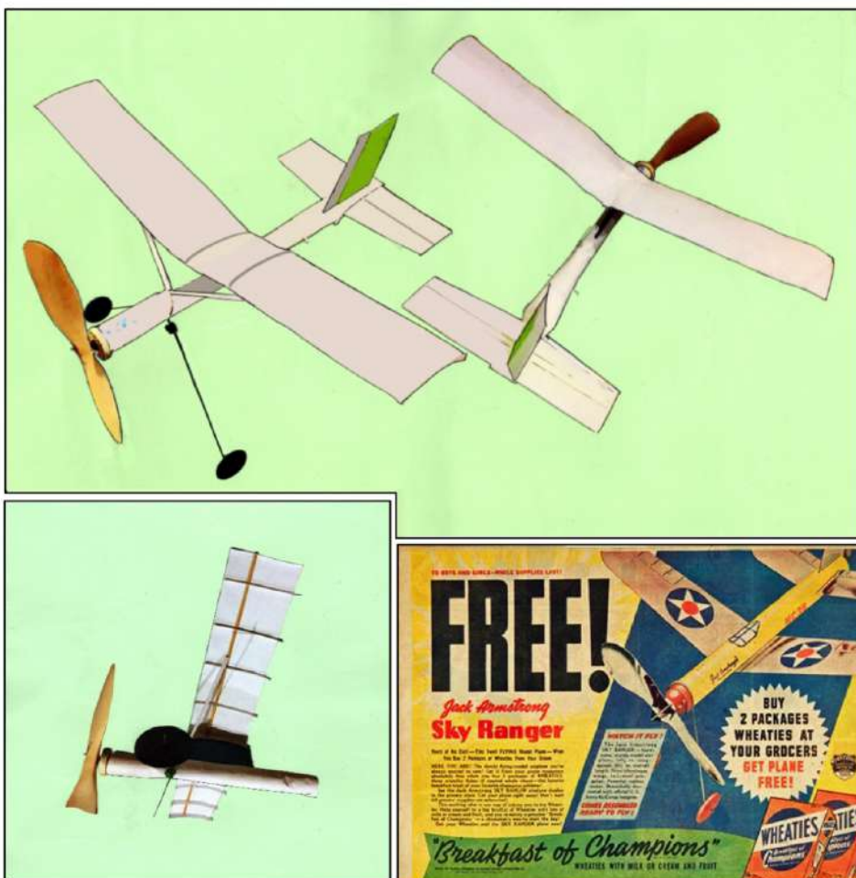
Fig 1: Brian's 'Mk II' contender Peterborough Rubber Powered Paper Plane Nationals (PRPPN). It has a wingspan of 18" with a 3" cord, its length is 14" and it weighs a smidgeon under 29 grams. It is powered by a single 20" loop off 1/8 rubber. Its best duration (with a limited number of turns) was a short, but promising, 12 sec. When putting this montage together I couldn't help noticing the model bears more than a little resemblance to the 'Sky Ranger' that came free with two packets of 'Wheaties' (bottom right). The advert is from, I would guess, the early 1950s.
