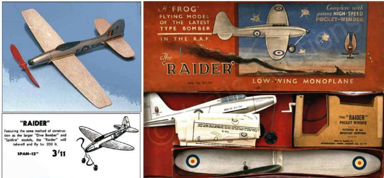
Fig 7: I was as thrilled with my FROG 'Fury' (top left) as Brian was with his larger and more sophisticated 'Raider'. The wings and tail of both models were thin balsa, but the preformed fuselages were made of card or paper, heat pressed in a hydraulic mould. These were light and, as they had to be in the hands of us young fledgling fliers, tough.
