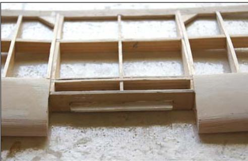
The centre section above the cabin is filled in with sheet. I have used 1.5mm sheet to allow for sanding to form. I will cut out the skylight, cover the centre section with film and add the glazing on the underside before gluing it into place. Once I have inserted the anchor points for the struts the wing will be ready for covering. I am using Toughlon which is a heat shrink covering material that has good adhesion and shrink-
