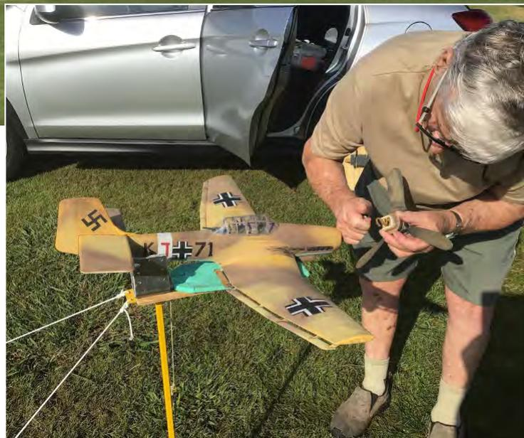
*TOP: The Stuka propellor made from moulded laminations of ply connected to the hub with flexible weed trimmer cord.*
